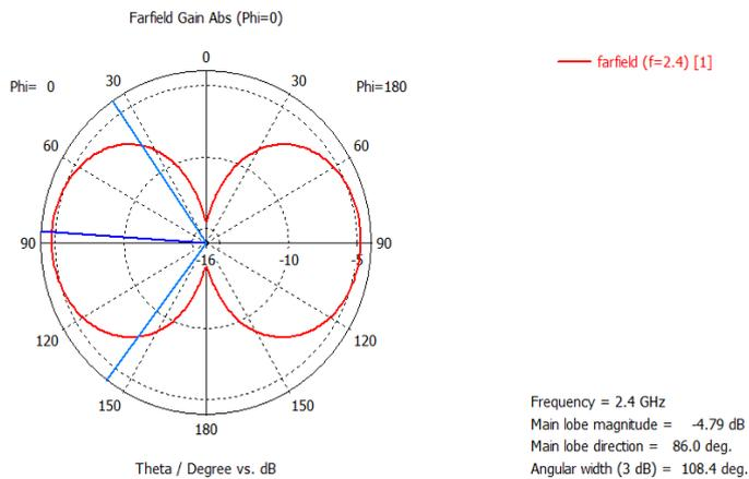
Fig -10: Gain of alumina substrate
