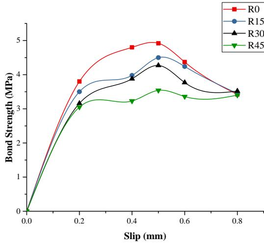
**Chart-4:** Bond Strength Vs Slip Curve of M.S. on 28 Days of Curing
