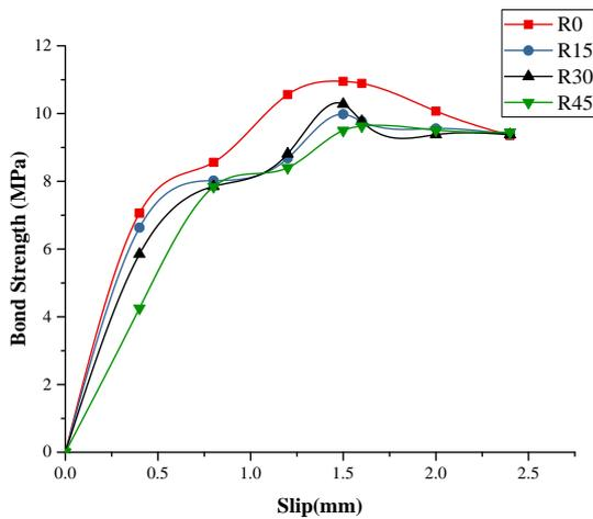
**Chart-10:** Bond Strength Vs Slip Curve of Fe500 on 28 Days of Curing
