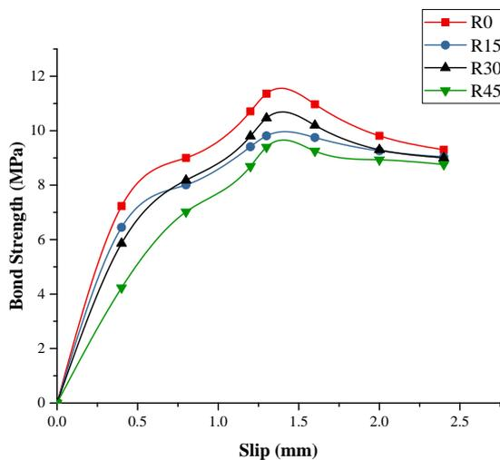
**Chart-6:** Bond Strength Vs Slip Curve of Fe415 on 7 Days of Curing
