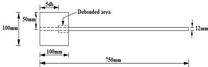
Fig- 1: Model of Pull-out Test Specimen
