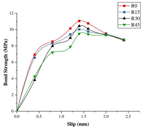
**Chart-9:** Bond Strength Vs Slip Curve of Fe500 on 7 Days of Curing
