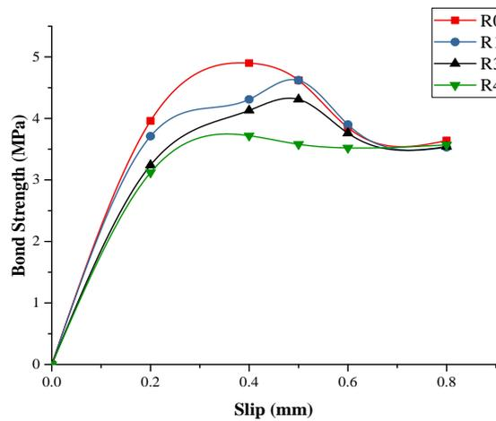
**Chart-5:** Bond Strength Vs Slip Curve of M.S. on 56 Days of Curing
