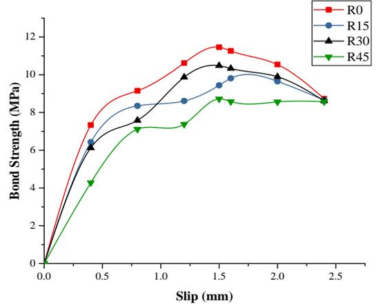
**Chart-8:** Bond Strength Vs Slip Curve of Fe415 on 56 Days of Curing
