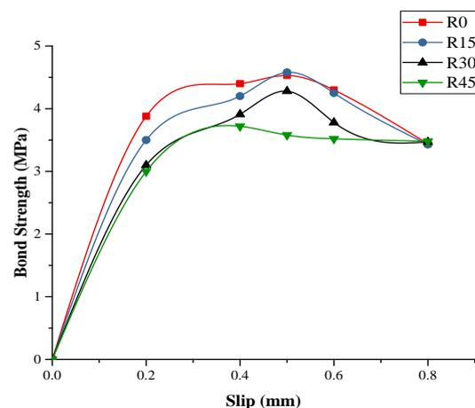
Chart-3: Bond Strength Vs Slip Curve of M.S. on 7 Days of Curing
