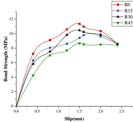
**Chart-7:** Bond Strength Vs Slip Curve of Fe415 on 28 Days of Curing
