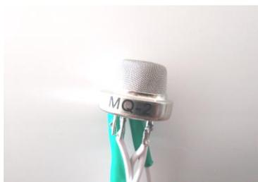
Fig -3: MQ2 Sensor
