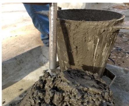
Fig. 3 Slump cone test of concrete
