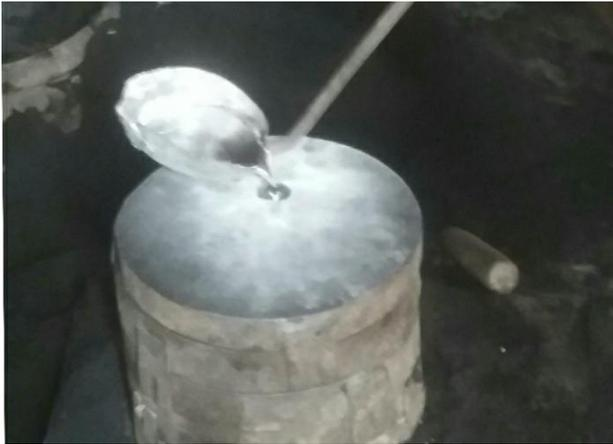
Figure-1: Casting of Aluminium Alloy
