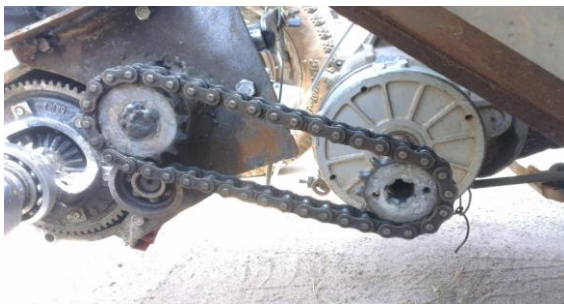
Fig. 19: Chain drive used in the vehicle
