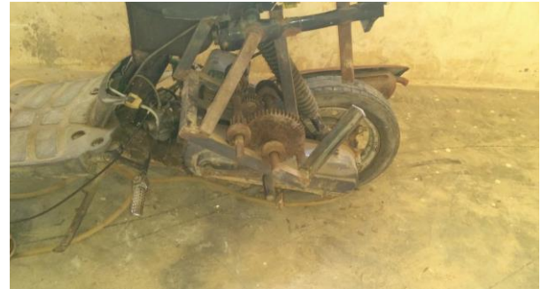
Fig. 21: Modified vehicle installed with reverse gear mechanism
