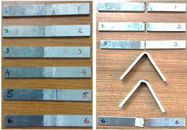
Fig. 6 Flexural specimen before test Fig. 7 Flexural specimen after test
