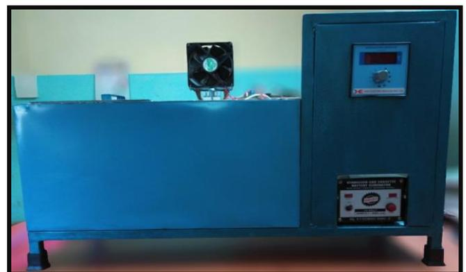
Fig.1 Fabricated setup of thermoelectric refrigerator
