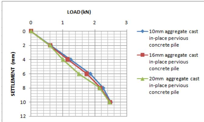
Chart-6: Behaviour of cast in-place pervious concrete piles.
