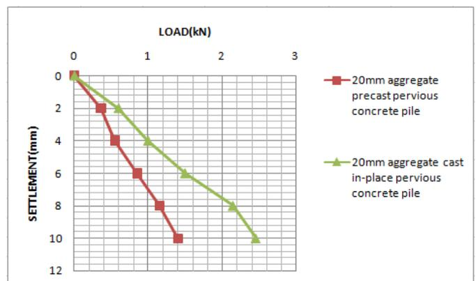
Chart-4: Load-settlement curve of 20mm aggregate piles.
