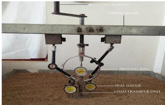
Fig-2: Loading setup
