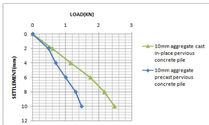
Chart-2: Load-settlement curve of 10mm aggregate piles.
