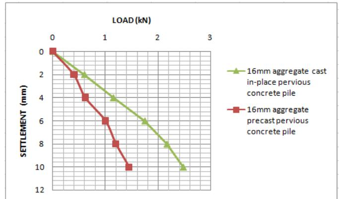
Chart-3: Load-settlement curve of 16mm aggregate piles.
