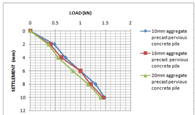
Chart-5: Behaviour of precast pervious concrete piles
