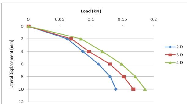
**Chart -7:** Load versus settlement curve for L/D= 40 and inclination= 45°
