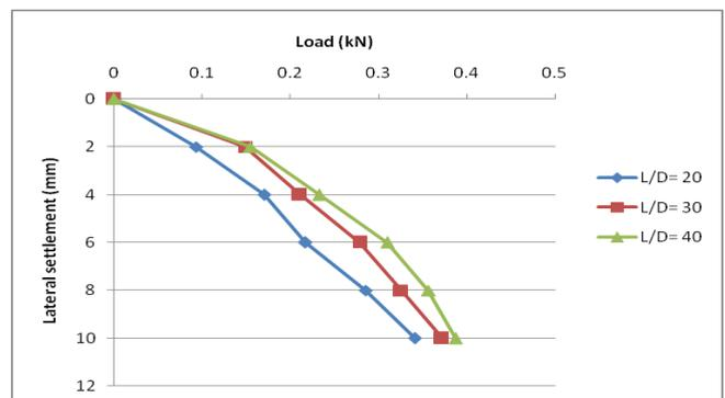
Chart -4: Load versus settlement curve for spacing= 2D and inclination= 15°
