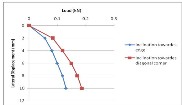
Chart -3: Load versus settlement curve for L/D=40, spacing= 4D and inclination= 45°
