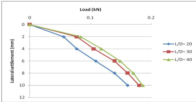
**Chart -5:** Load versus settlement curve for spacing= 4D and inclination= 45°
