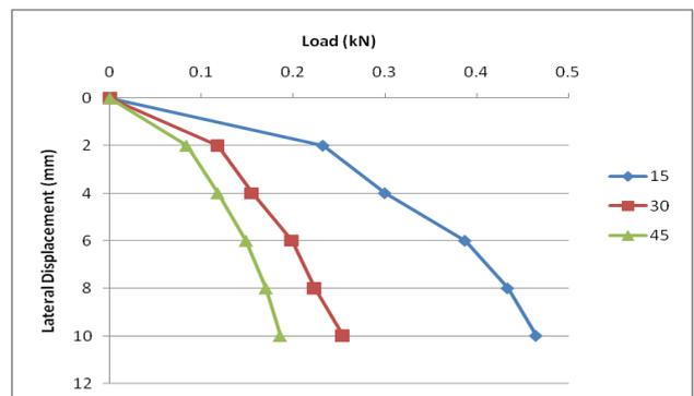
**Chart -9:** Load versus settlement curve for L/D= 40 and spacing= 4D
