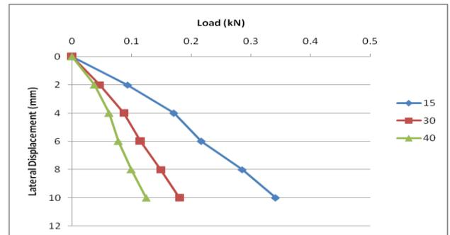
**Chart -8:** Load versus settlement curve for L/D= 20 and spacing= 2D
