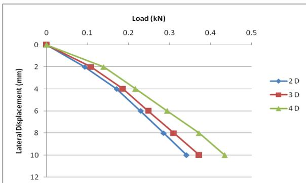
**Chart -6:** Load versus settlement curve for L/D= 20 and inclination= 15°
