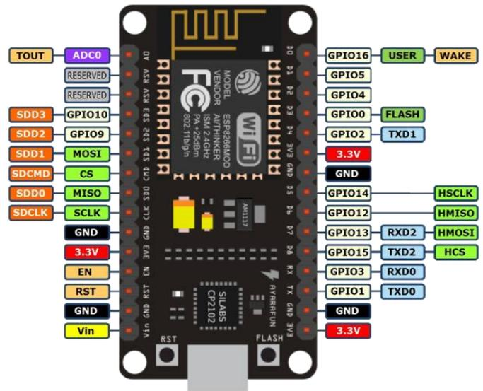
Fig -1: ESP 8266 Pin Diagram
