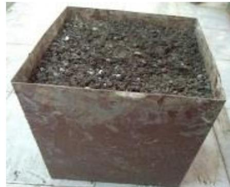
Fig -4: Soil filled in the Mini Plate load tank
