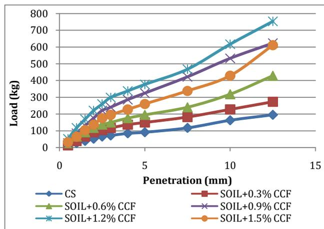
**Chart -3:** Load Penetration curve of soaked CBR test for soil specimen with varying percentage of CCF
