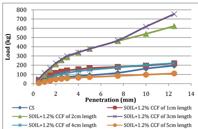
**Chart -7:** Load Penetration curve of soaked CBR test for soil with 1.2 % CCF of varying lengths
