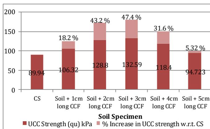
Chart -6: UCC strength and percentage increase in UCC strength for soil with 1.2 % CCF of varying lengths
