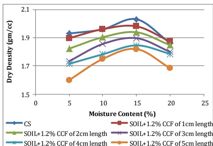
Chart -5: Graph of Moisture content v/s Dry Density for soil specimens with varying lengths of CCF
