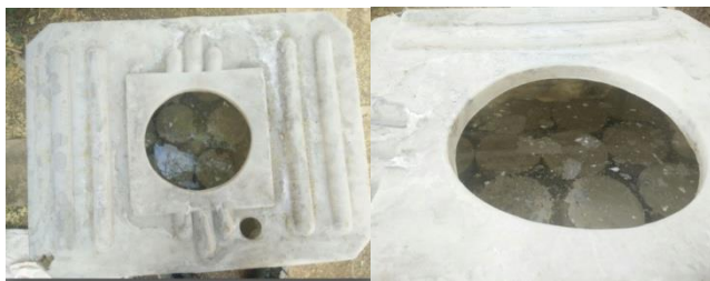
Fig 11: Specimens Placed in 2.8M NaCl Solution
