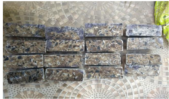
Fig 13: Specimens treated with AgNO 3 Solution
