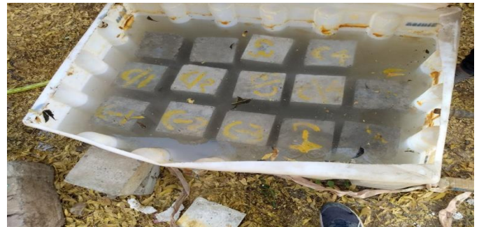
Fig 8: Curing of Specimen in Sulphuric Acid (day 0)
