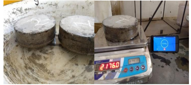
Fig 3: Sorptivity Test Setup
