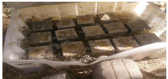
Fig 8: Curing of Specimen in Sulphuric Acid (day 28)
