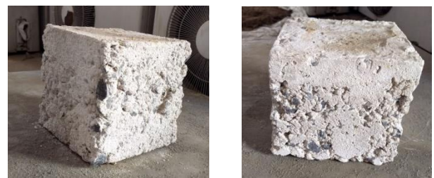
Fig 9: Degradation of Specimen after Acid Curing
