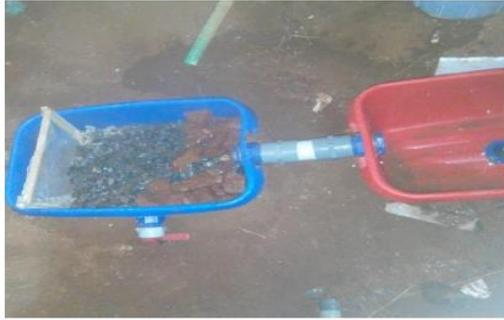
Fig 3.4 Oil retaining wooden baffle
