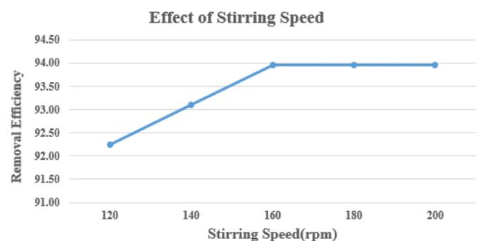
Fig.4 Stirring Speed on RHA Adsorbent
