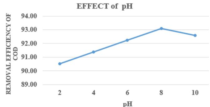
Fig.3 pH on RHA Adsorbent
