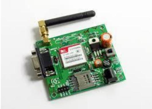
**Fig:3 GSM modem**
