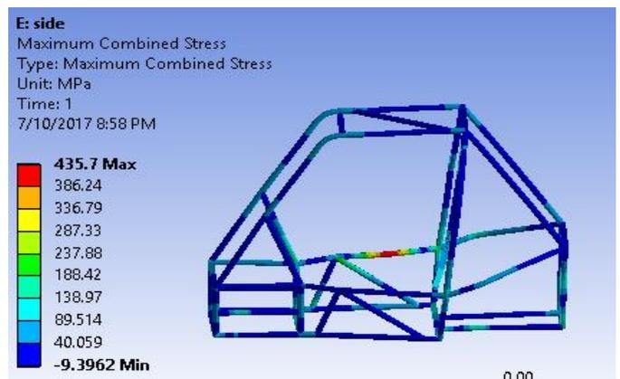
Figure 7: Maximum Stress in Side Impact
