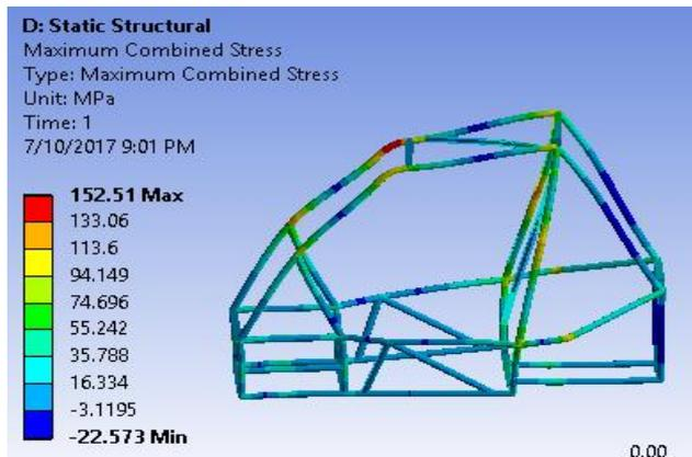
Figure 9: Maximum Stress in Roll Over
