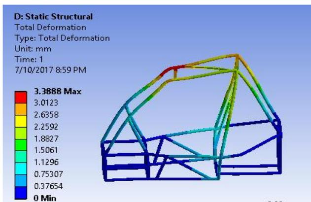
Figure 10: Maximum Deformation in Roll Over
