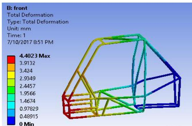
Figure 4: Maximum Deformation in Front Impact
