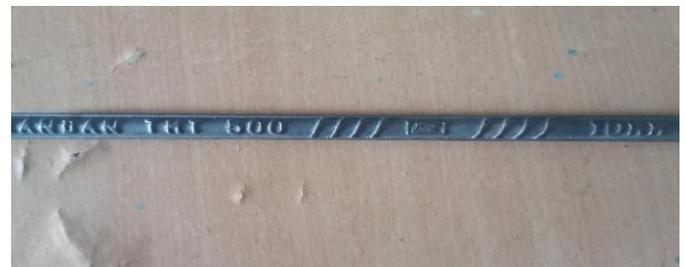
Fig -2: Reinforcement Steel Bar (Before Corrosion)
