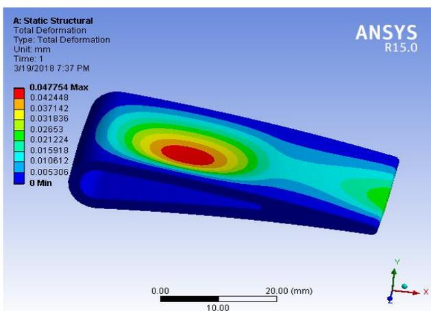
Fig-7: Total Deformation for material of Titanium T6
