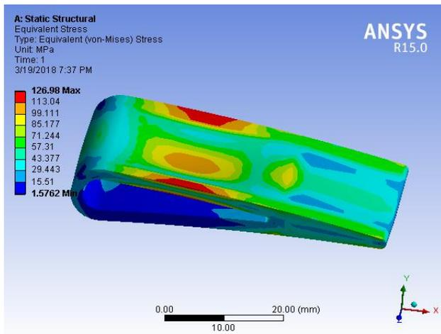
Fig-6: Total Von Misses Stress for material of Titanium T6
