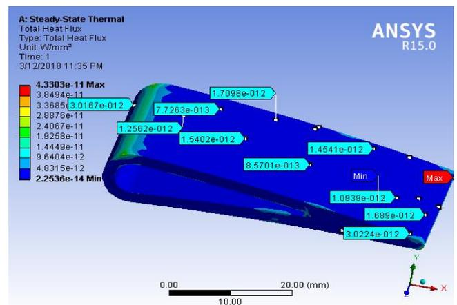
Fig -4: Total heat flux for sic
