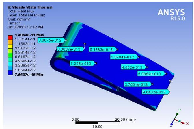
Fig -3: Total heat flux for titanium t6
