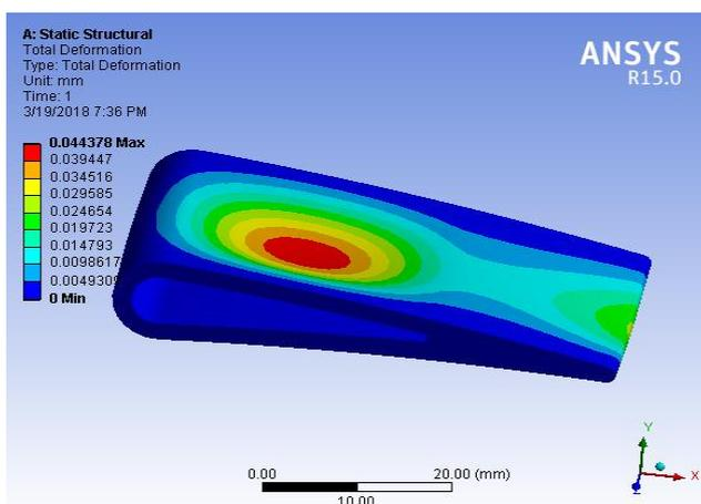
Fig -8: Total Deformation for material of SIC
