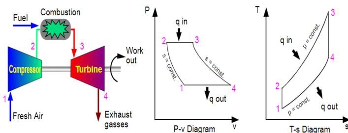
**Fig-1** : working of Brayton cycle
