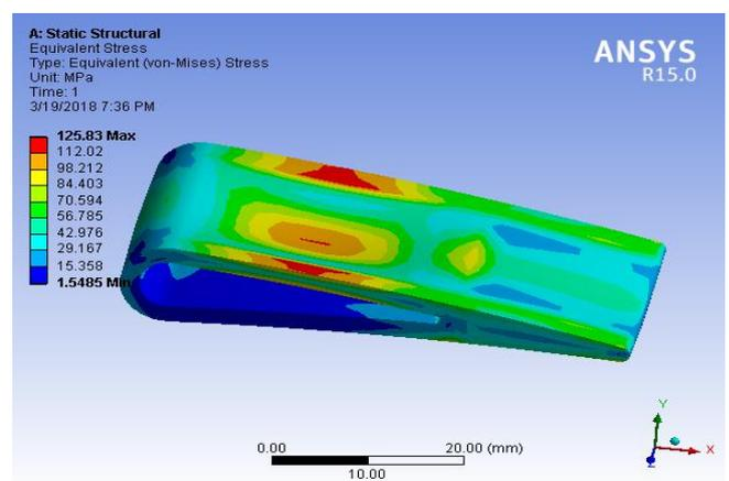
Fig -5: Total Von Mises Stress for material of SIC
