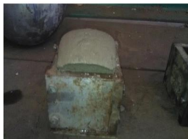
FIG 2.2. CONCRETE MIX AFTER ADDITION OF Al POWDER
