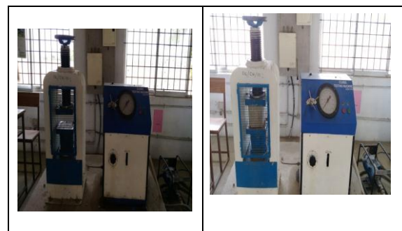
Fig 4: Compression testing on cube specimen
