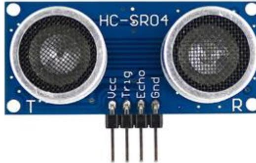
The ultrasonic sensor used here performing function of continuous monitoring of surrounding To detect an obstacle such as human, animals etc. The ultrasonic sensor basically works on principal of SONAR.
