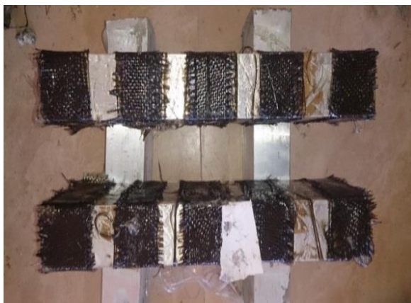
Fig -3: Retrofitted ATC sample
