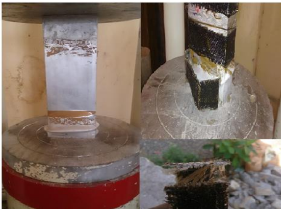
Fig -5: Elephant's Foot Buckling, Buckling Fold & Ruptured BFRP
