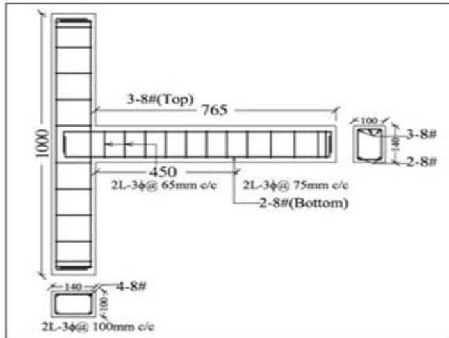
**Figure 3:** Dimension and reinforcement details of control specimens
