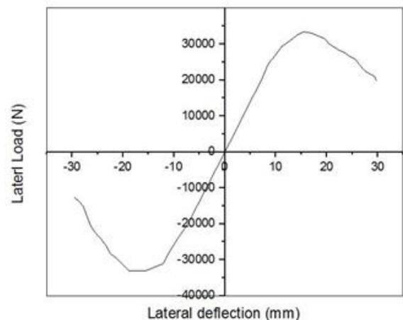
Figure 12: Lateral Load vs Lateral Deflection: PUG
