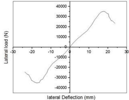
Figure 10: Lateral Load vs Lateral Deflection: H-lam
