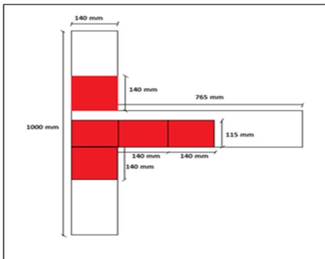
**Figure 4:** Configuration of panel wrapping
