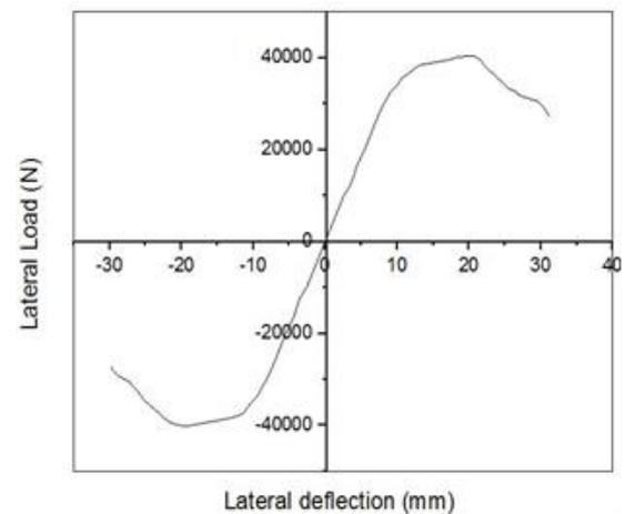
Figure 11: Lateral Load vs Lateral Deflection: I lam
