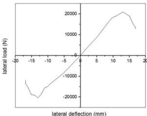
Figure 9: Lateral Load vs Lateral Deflection: BCJ - CS
