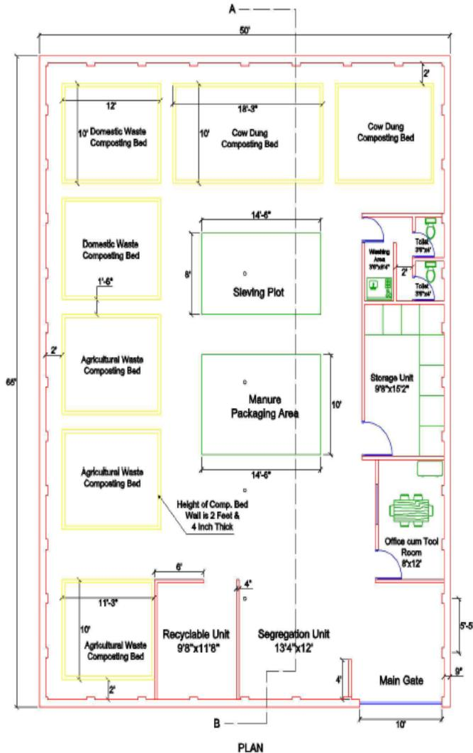
Fig 4: Plan, Elevation & Section for SWM
