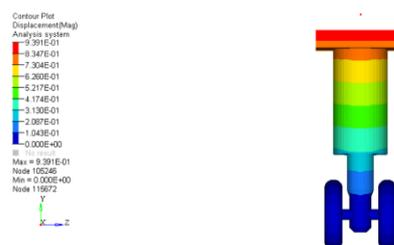
First mode shape of Landing gear system.
