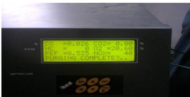
**Fig.-1 Netel exhaust gas analyser**
