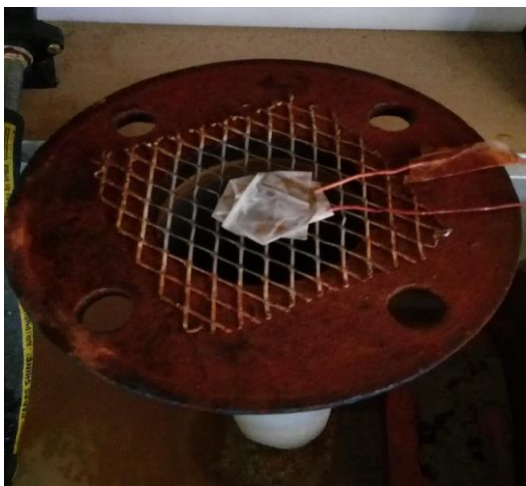
Figure 4 (b) Housing of PZT-patch inside the flange coupling
