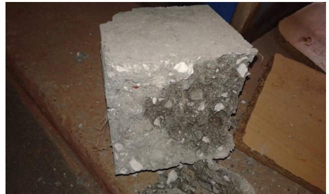
Fig 3- compressive strength test
