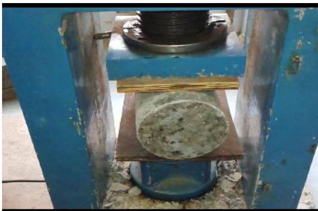
Fig 6- split tensile test
