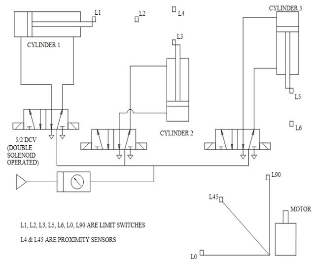
Fig -3: Operation of Pneumatic circuit.
