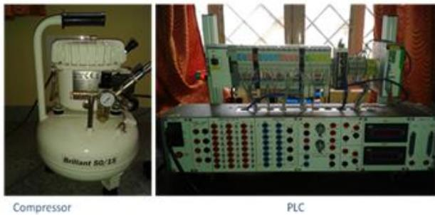
Fig -1: components used for setup
