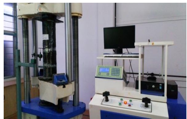
Fig.8 Universal Testing machine with specimen
