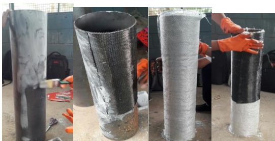
Fig.5 FRP wrapping with HCS column
