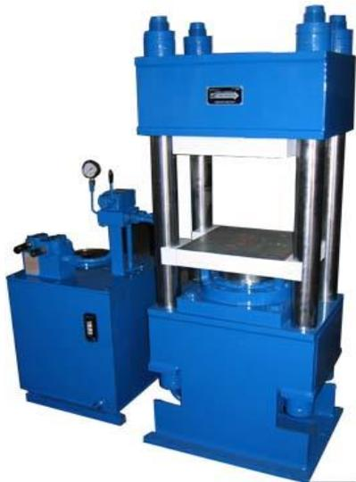
Figure 1 Compression Molding machine
