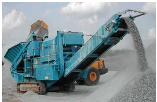
Mobile recycling plant
