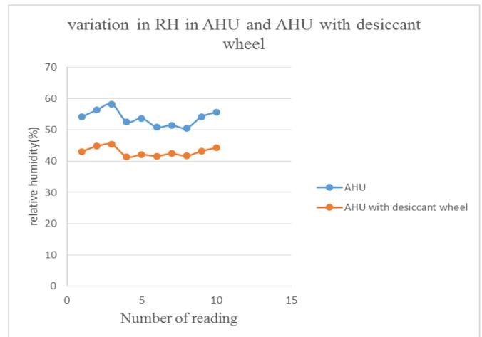
**Fig -2:** Variation of RH in AHU and AHU with desiccant wheel
