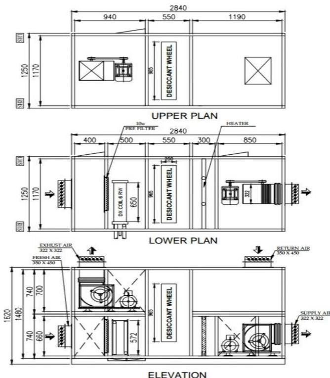
Fig -1: AHU with Desiccant Wheel
