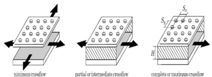
Fig -3: Definition of crossflow schemes in multi-jet systems (according to [57])
