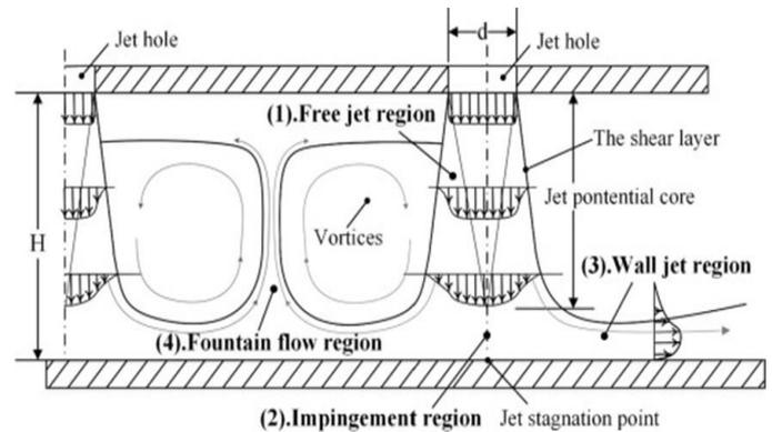
**Fig -2:** Multi jet impingement system.
