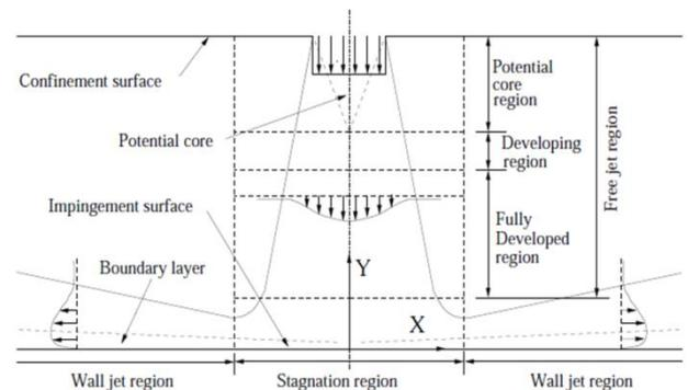
**Fig -1:** Schematic diagram of an impinging jet.
