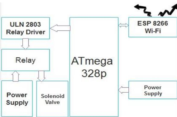
Fig 3: Valve Controlling Node
