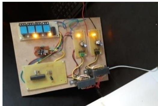
Fig 7: Valve Controlling Node
