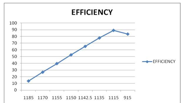
Fig. Efficiency Vs Speed Characteristics
