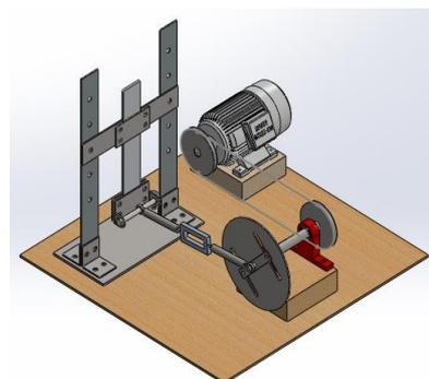
**Fig -3:** Third concept of the fatigue testing machine
