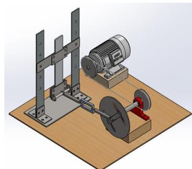
**Fig -3:** Third concept of the fatigue testing machine
