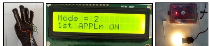
Fig-10: Switching ON first Appliance.
