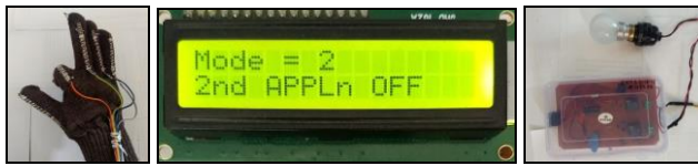
Fig-13: Switching OFF second Appliance.
