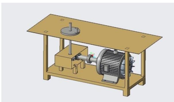
Bar bending machine is consist of electric motor, coupling, circular plate, worm gear drive, extended shaft. Electric motor transmits power to gear box where speed
