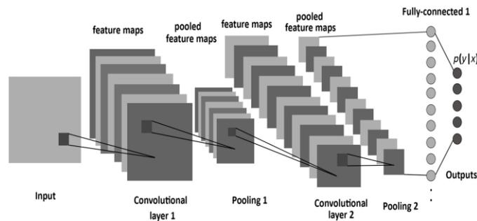
Figure 1: CNN Architecture
