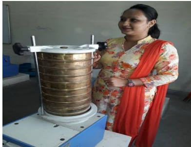
Fig: 2 Sieve analysis of fine aggregate (Sand)
