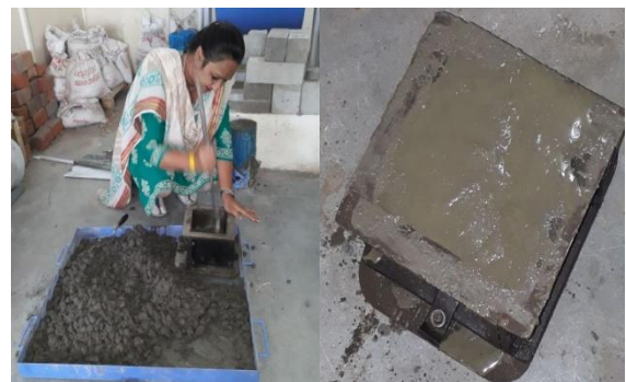
Fig: Mixing material and Filling of cubes
