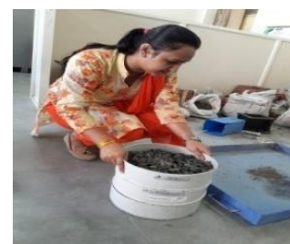
Fig: 1 Sieve analysis of coarse aggregate
