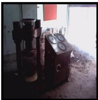
Fig 4.7: Compressive Strength Test
