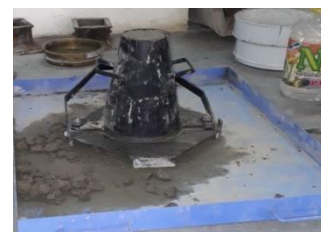
Fig: 4.6 Slump Cone test
