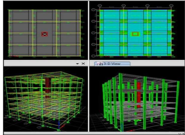
Fig -2: Plan of the Building with Shear Wall at the Center
