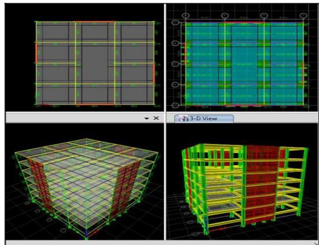
Fig -4: Plan of the Building with Shear Wall at the Edges
