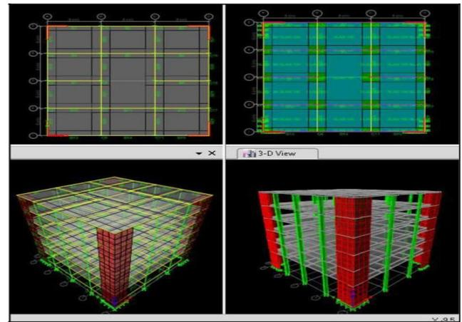
Fig -3: Plan of the Building with L - Shaped Shear Wall
