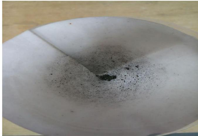
After heating the aqueous silver nanopowder it converts from semi liquid state to solid state. The solid state powder is need to be collected as shown in the figure.
