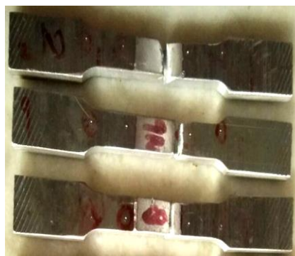
Fig 6. Tensile specimen after fracture
