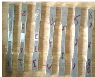
Fig 6. Tensile specimen after fracture
