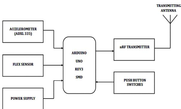
Figure 1: Block Diagram of Transmitter
