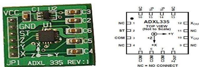
Figure 2: Accelerometer (ADXL 335)
