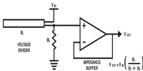
Figure 4: Circuit Diagram of Flex Sensor
