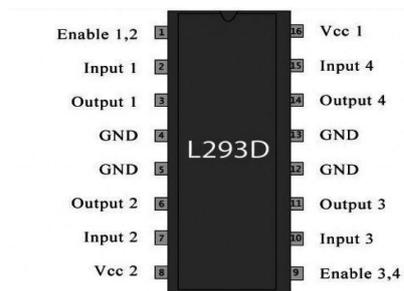
Figure 6: Pin Diagram of L293D IC
