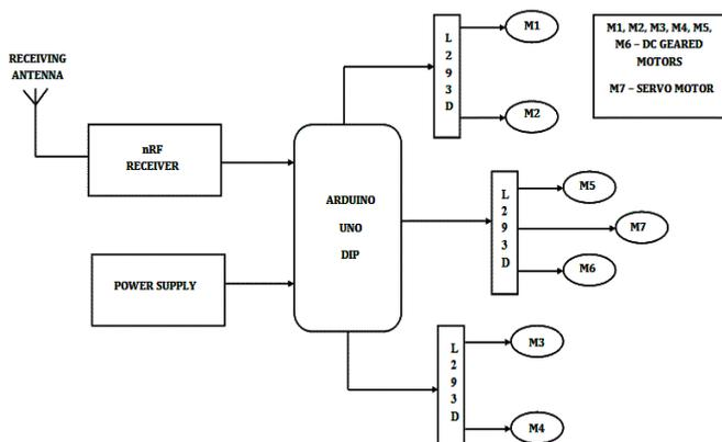
Figure 5: Block Diagram of Receiver
