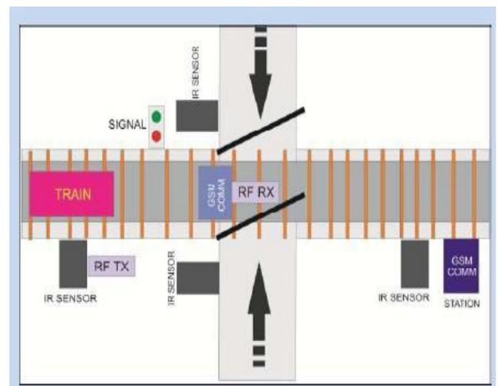
Figure 1.3: Automated Railway Crossing System [10]
