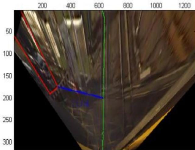
Figure 2.5: Subplot shows the bird's eye view of detected vehicle, marked in red box [2]
