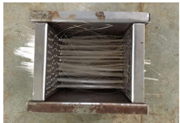
Figure 4: A special Hollow mould I made by my self so I can place good amount of Optical fibers uniformly.
