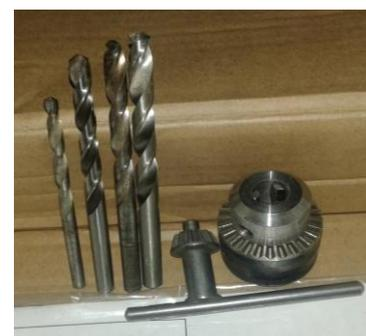
**Fig -9:** Drill tool & Chuck
