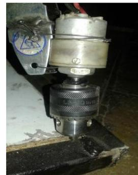
**Fig -8:** Motor & Chuck
